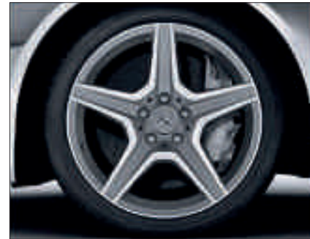
AMG 5-spoke light-alloy wheels with 235/40 R 18 front tyres and 255/35 R 18 rear tyres, painted in titanium grey with a high-sheen finish (optional for C 63 AMG, Code 790).
