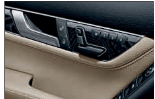
The Memory package remembers up to three positions for the driver's seat, steering column and exterior mirrors.
