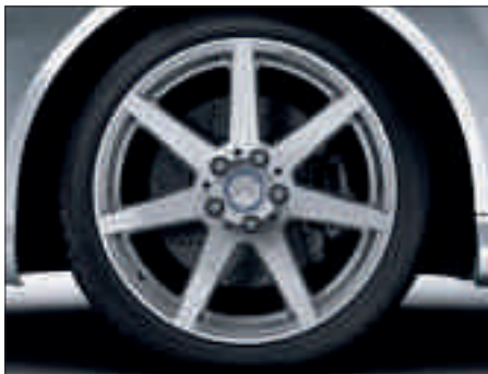
AMG 7-spoke light-alloy wheels with 225/40 R 18 front tyres and 255/35 R 18 rear tyres, with a high-sheen finish (optional, not for C 63 AMG, Code 782).
