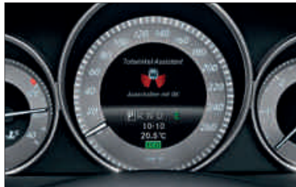
Active Blind Spot Assist monitors the difficult-to-see areas to the left and right of the car.
