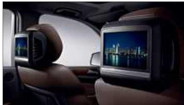
The two displays for the Rear Seat Entertainment System are mounted on the front-seat head restraints.
