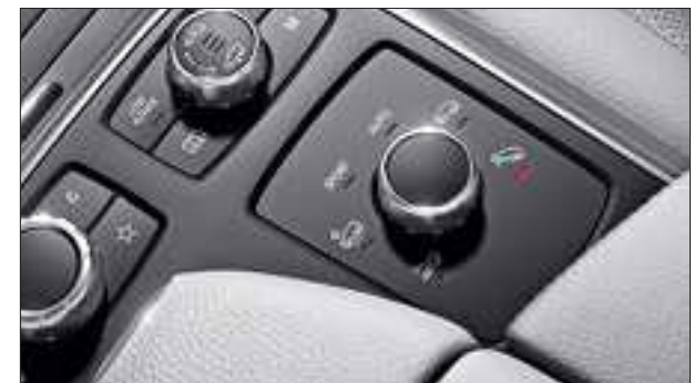
A rotary switch in the centre console is used to set the current driving mode.
