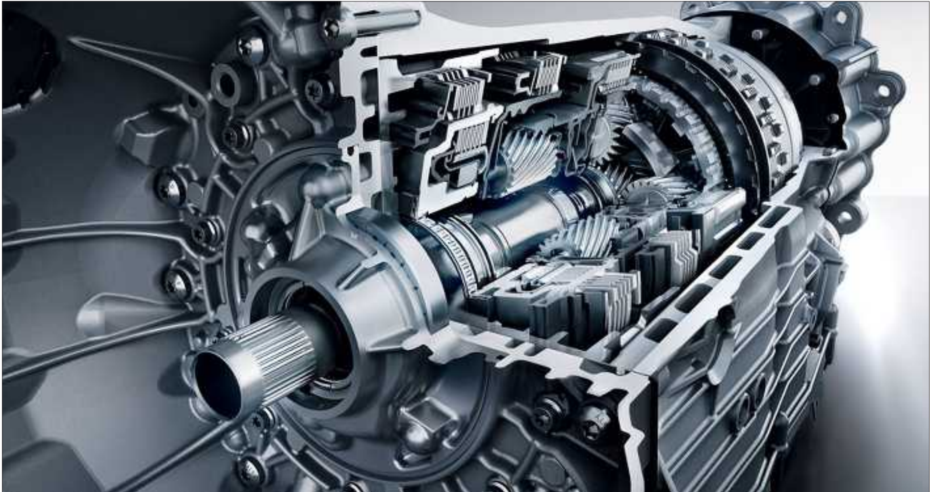
The automatic transmission 7G-TRONIC PLUS: one of over 18 million Mercedes-Benz automatic transmissions produced in a period spanning more than 50 years.
