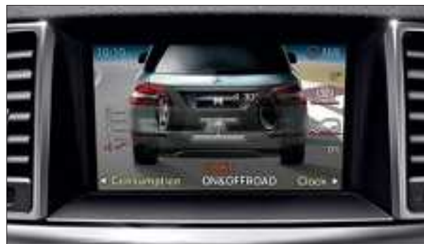
The COMAND display shows the driving mode as well as the gradient and angle of inclination.
