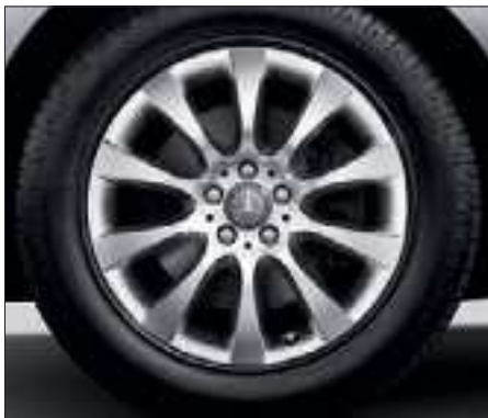
10-spoke light-alloy wheels with 255/55 R 18 tyres (standard for ML 350 4MATIC, optional for diesel models, Code R41).
