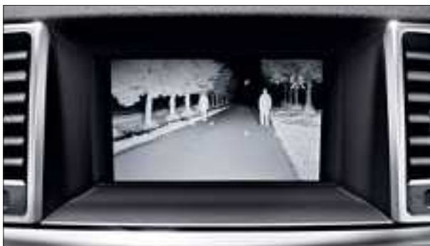
To ensure better driver awareness, Night View Assist Plus highlights pedestrians on the display.
