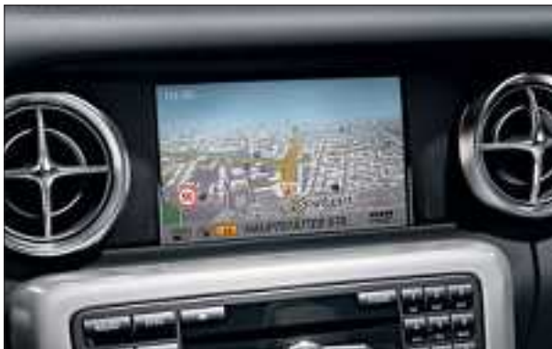
The information from Speed Limit Assist is shown both in the instrument cluster and in the COMAND Online central display.
