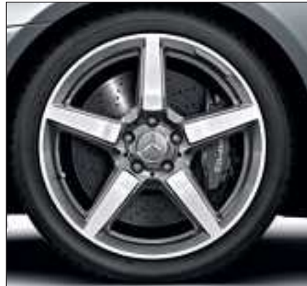
5-spoke AMG light-alloy wheels, painted titanium grey with a high-sheen finish, with 235/40 R 18 front and 255/35 R 18 rear tyres (standard for SLK 55 AMG, Code 790).
