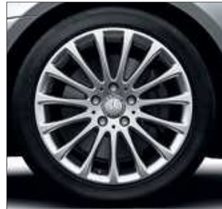
Multi-spoke light-alloy wheels with 225/45 R 17 front and 245/40 R 17 rear tyres (option, Code R81).
