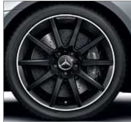
10-spoke AMG light-alloy wheels, painted black, high-sheen rim flange, with 235/40 R 18 front and 255/35 R 18 rear tyres (option, Code 760).
