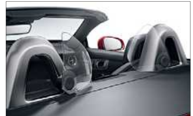
The draught-stop system AIRGUIDE minimises draughts in the interior of the open vehicle.
