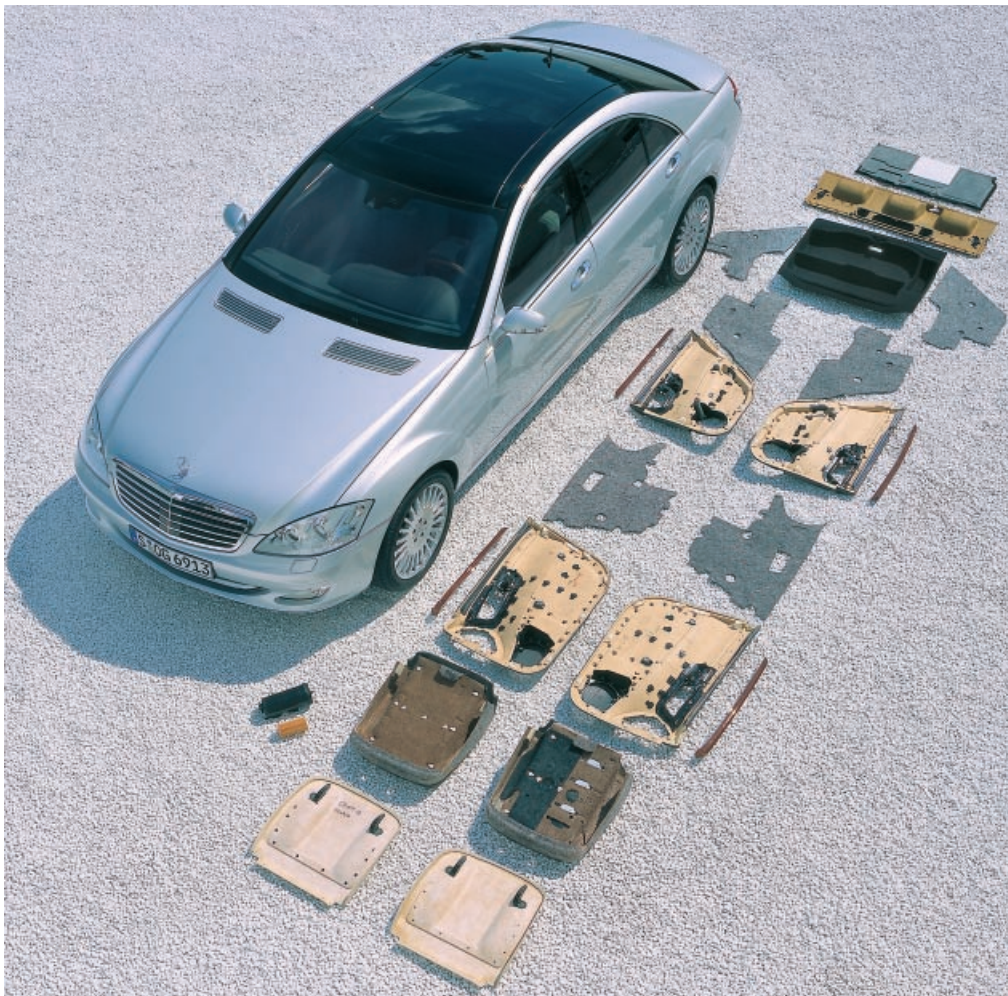
Abbildung 4-12: Bauteile aus nachwachsenden Rohstoffen in der S-Klasse Figure 4-12: Components of the S-Class made of renewable raw materials
