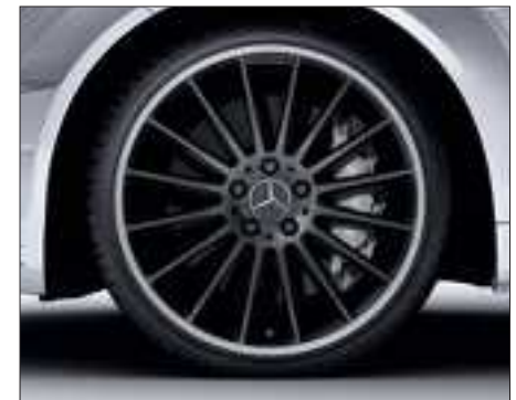
Multi-spoke AMG light-alloy wheels, painted matt black, rim flange with a high-sheen finish, with 235/35 R 19 front tyres and 255/30 R 19 rear tyres (optional for C 63 AMG, Code 797).
