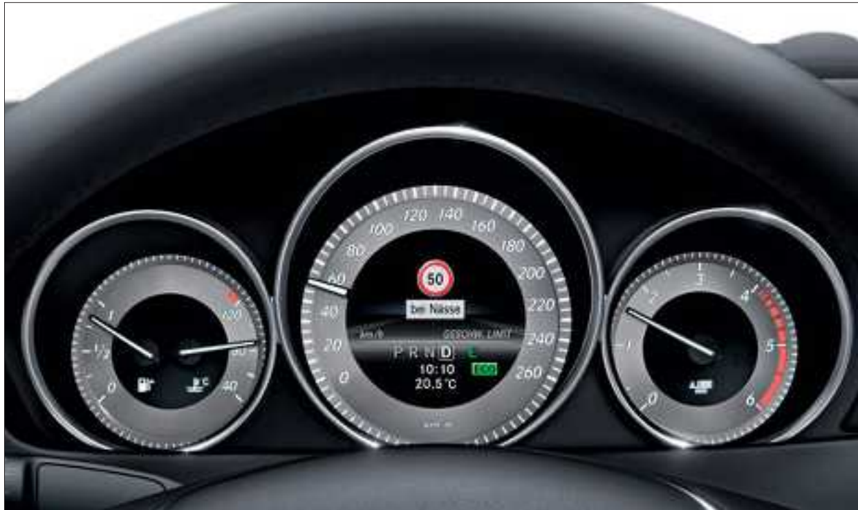
Speed Limit Assist shows the driver the current speed limit.
