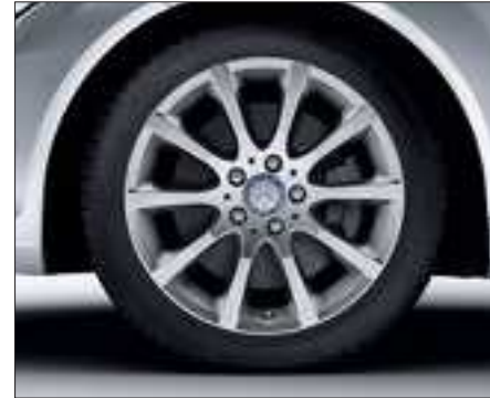
10-spoke light-alloy wheels with 245/45 R 17 tyres (standard for C 200, C 250 CDI, C 250 and C 350, Code 25R).
