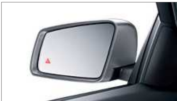
Blind Spot Assist can warn of potential dangers acoustically and by means of a red warning triangle in the exterior mirror.
