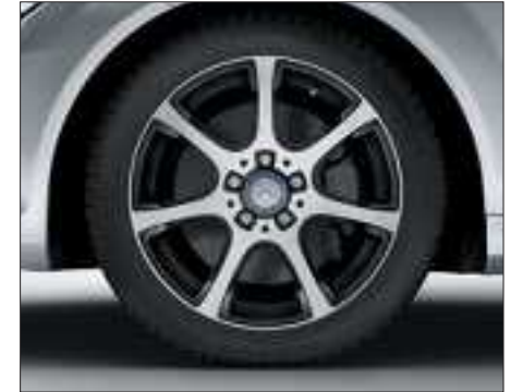
7-spoke light-alloy wheels with 225/45 R 17 front tyres and 245/40 R 17 rear tyres, painted high-gloss black with a high-shine finish (optional, Code 74R).
