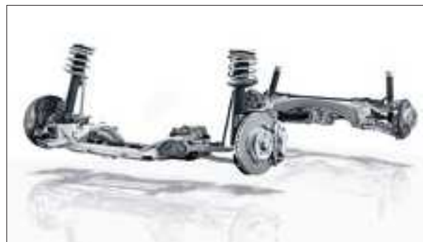
A suspension system lowered by 15 millimetres is one of the features which complements the Dynamic Handling package.
