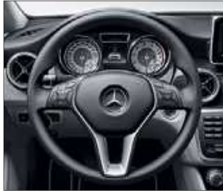
12-button three-spoke multifunction steering wheel
