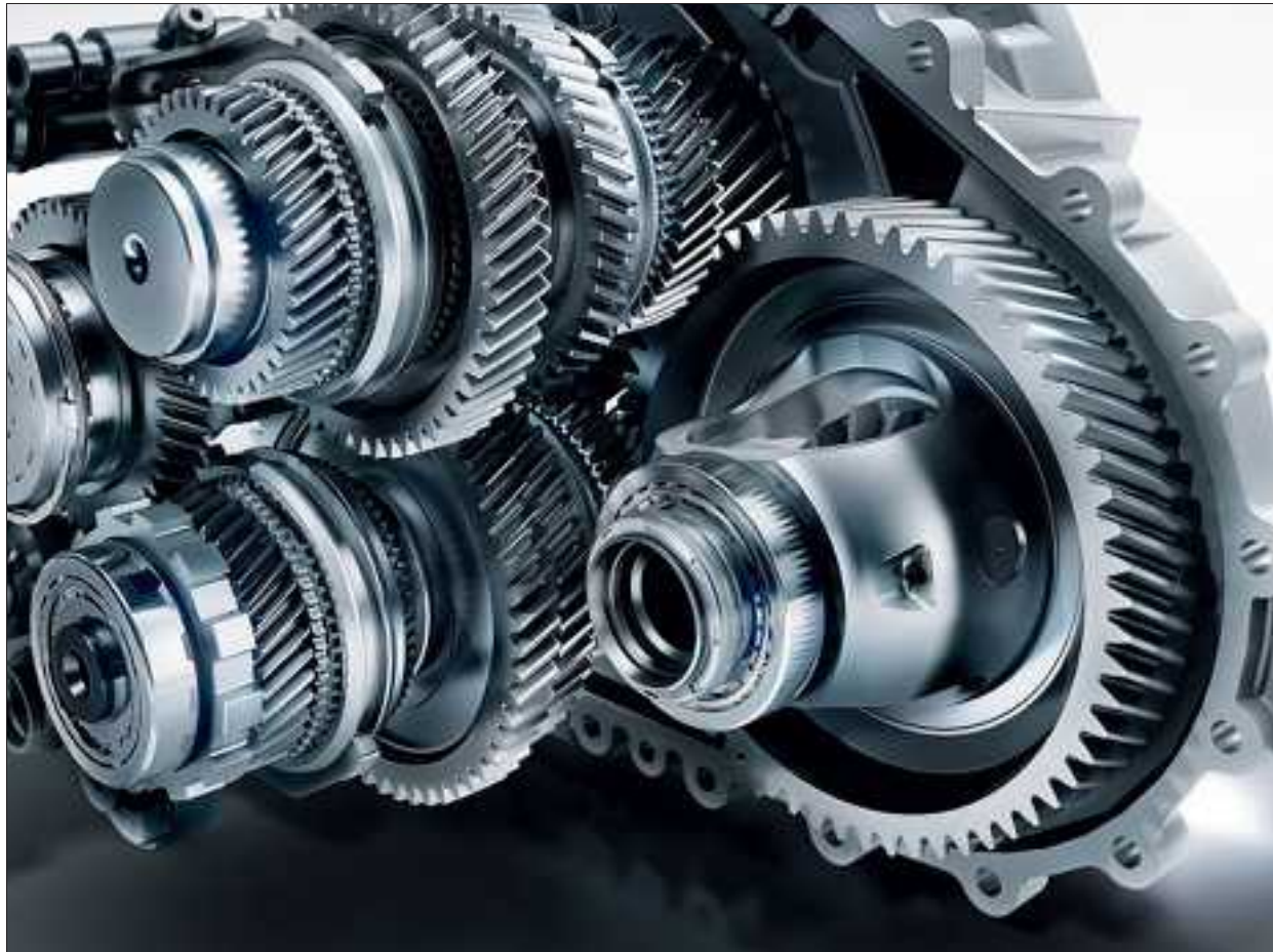
The 7G-DCT seven-speed dual clutch transmission enables gear shifting without any interruption in tractive power
