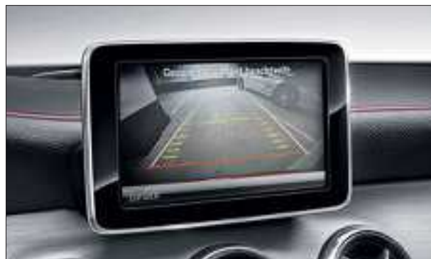
The reversing camera supports the driver when backing into a parking space. It is available in combination with Audio 20 CD and COMAND Online
