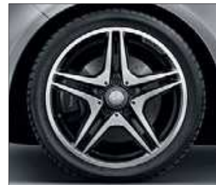
AMG 5-twin-spoke light-alloy wheels with 225/40 R 18 tyres, painted black with a high-sheen finish (option, Code 781)
